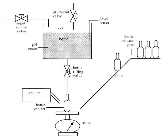
Figure 5: the physical structure of the bottle filling plant, excluding the supervisor and the operator interfaces. Only one bottle filling line is shown.
